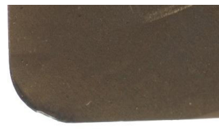
Tool wear after 30 hours of machining
